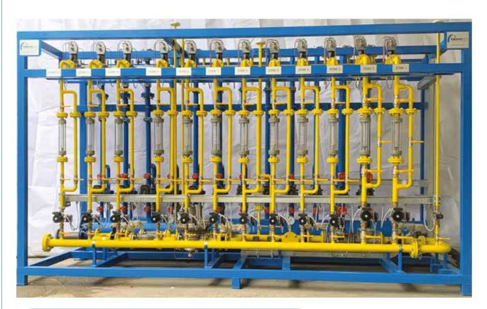
Thanks to AQRatio technology the air/gas ratio is kept constant during the regulation output driven by the temperature profile demand and it is independent from the pressure losses in the air/gas mixture line downstream the regulation skid due to any cause (to fouling in the pipe or in the burners).
